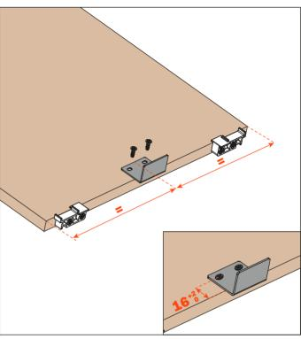
2) Fixing the magnet to the bottom.
