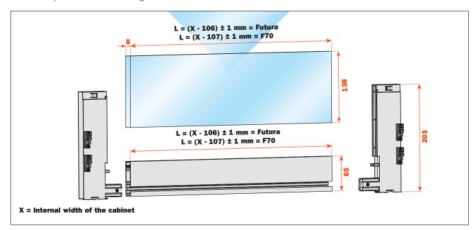
Insert the front panel adapters into the front panel and tighten the locking screws. Frontal fixings are already premounted.
