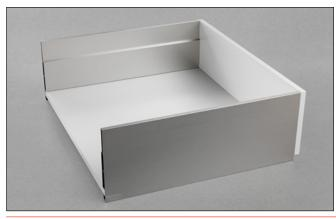
Lineabox metal sides, wooden bottom and back panel. Height of the side 178 mm - Internal height 149 mm. For use with F70 and Futura full-extension runners.
