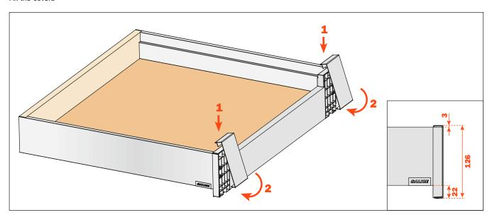
To correct any possible cutting errors of the panel, loosen and retighten the indicated screws
