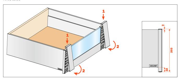
To correct any possible cutting errors of the panel, loosen and retighten the indicated screws
