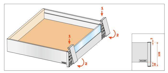
To correct possible cutting errors of the panel, loosen and retighten the indicated screws
