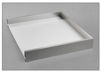
Lineabox metal sides, wooden bottom. Height of the side 75 mm - Internal height 46 mm. For use with F70 and Futura full-extension runners.
