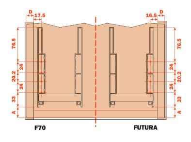
Dimensions and drilling of the internal frontal
