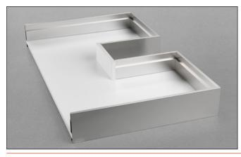
Lineabox metal sides, wooden bottom. Height of the side 101 mm - Internal height 72 mm. For use with F70 and Futura full-extension runners.
