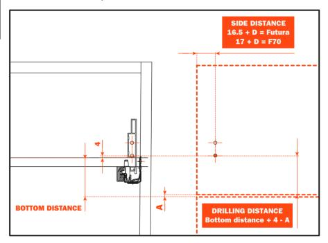
Once the pilot drilling position is set, proceed with the other pilot drillings according to the Lineabox side template used for this drawer. Attach the drawer front and proceed with all the remaining drawers.
