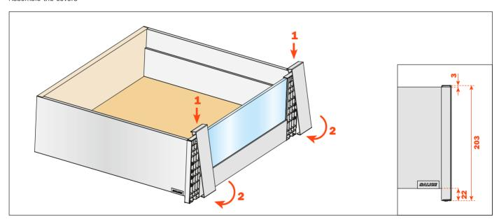
To correct any possible cutting errors of the panel, loosen and retighten the screws as shown
