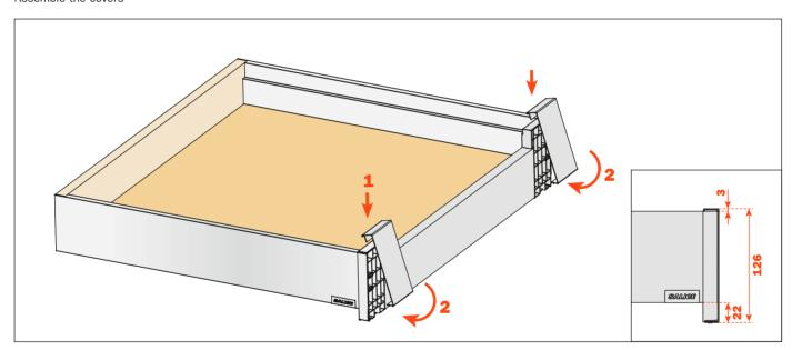
To correct possible cutting errors of the front profile, loosen and retighten the screws as shown
