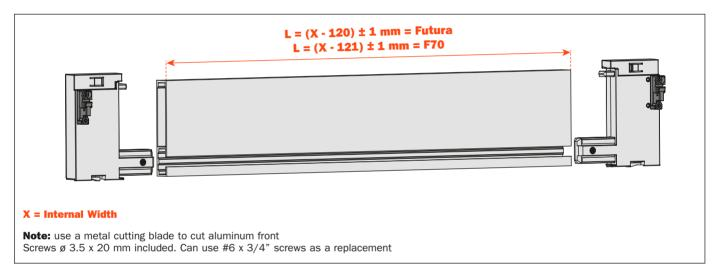
Insert the front panel adapters into the front panel and tighten the locking screws. Front clips are already premounted.
