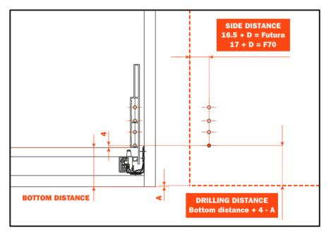
Once the pilot drilling position is set, proceed with the other pilot drillings according to the Lineabox side template used for the first drawer. Attach the drawer front and proceed with the upper drawer.
