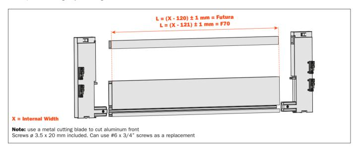
Insert the front panel adapters into the front panel and the railing and tighten the locking screws. Front clips are already premounted.
