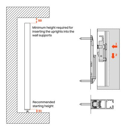
Wall fixing of the first upright profile and location of the supports We suggest that the parallelism between the slots is checked by inserting 2 brackets For the perfect alignment of the upright profiles see the chapter "Adjustments"
