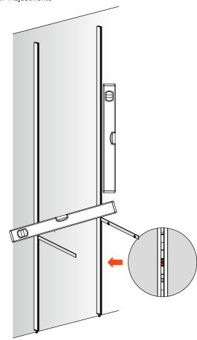
before fixing the upright profile to the wall, check the accessibility of the adjustment screws and the correct alignment between the upright profiles
