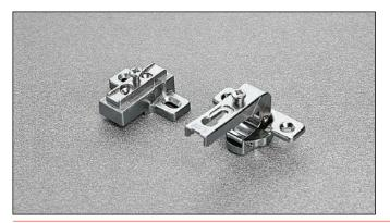
Crampon hinges. For smaller spaces with 15x32 mm drilling. 11.5 mm deep metal cup. 94° opening. Possible drilling distance on the door (K): from 3 to 8 mm. Compatible with all traditional Series 200 mounting plates, 28x32 mm drilling.
