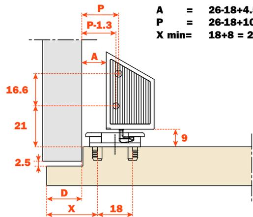
$$\begin{aligned} A &= X - D + 4.5 \\ P &= X - D + 10.8 \\ X \text{ min} &= D + 8 \end{aligned}$$
