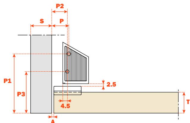
$$\begin{aligned} P &= 14.8 + A \\ P1 &= 36.8 + T \\ P2 &= P - 1.3 \\ P3 &= P1 - 16.5 \end{aligned}$$
