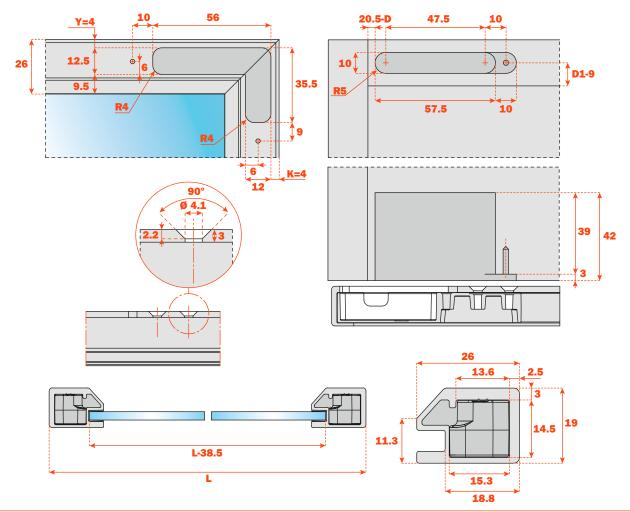
Formulas to determine the distance for the insertion of the holders for arm.
