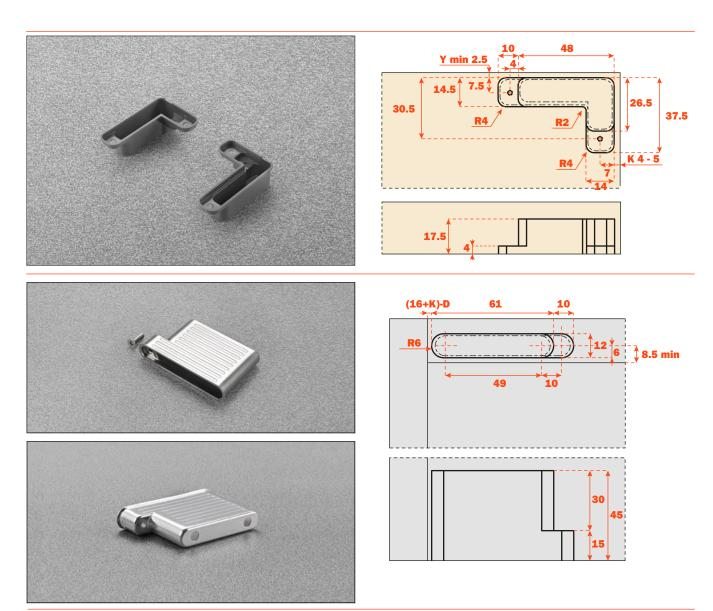
Formulas to determine the distance for the insertion of the holders for arm.
