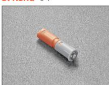
Optional supplementary release device to increase the magnetic holding strength. It must always be used together with the DPM. The suggested position of the DPM is the point of pressure on the door. The DPA can be positioned at any point along the opening edge of the door.  $\emptyset$  10 mm, 40 mm length.
