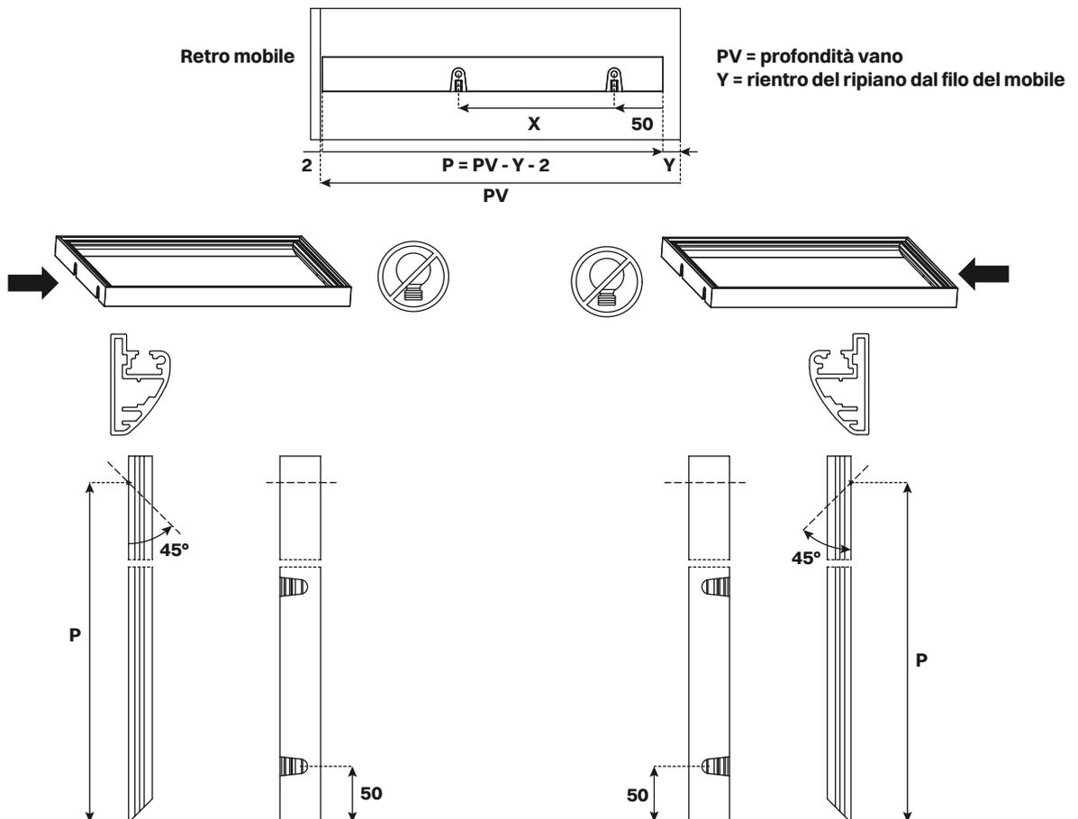
ASSEMBLAGGIO DEL RIPIANO SENZA LED
