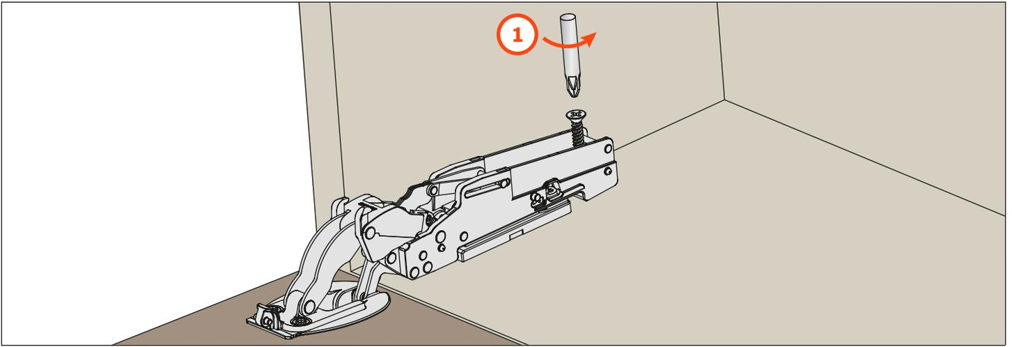
Un-snap the hinge from the mounting plate with a screwdriver
