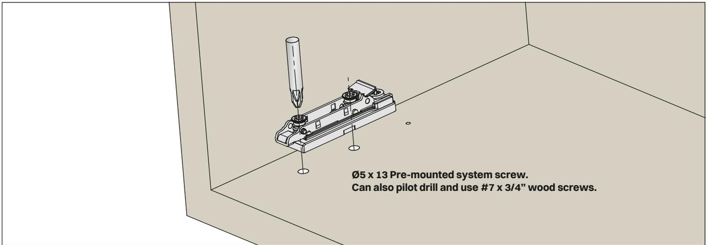
Attaching the hinge to the door
