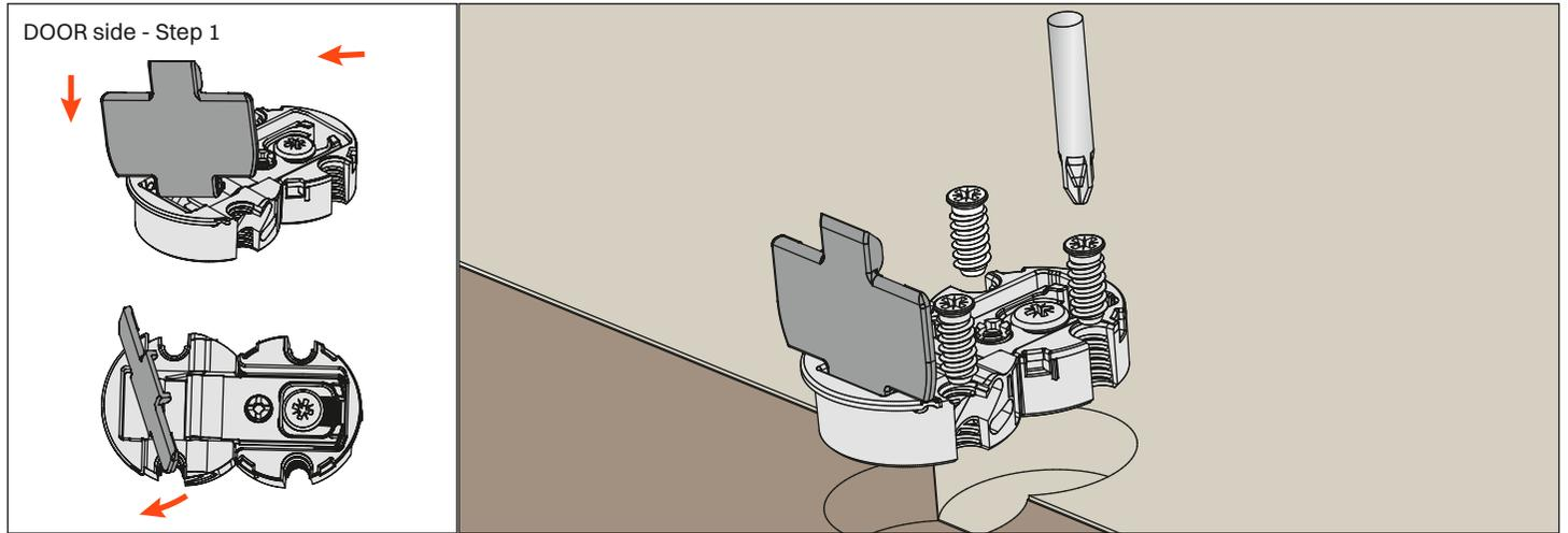
After attaching the hinge, make any adjustments required.
