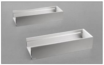
Lineabox Easy metal sides, wooden bottom and back panel. Height of the side 101 mm - Internal height 72 mm. For use with Progressa and Futura full-extension runners.
