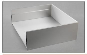
Lineabox Easy metal sides, wooden bottom and back panel. Height of the side 178 mm - Internal height 149 mm. For use with Progressa and Futura full-extension runners.
