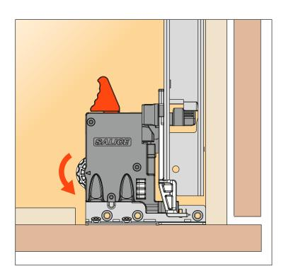
Rotate the white wheel (see drawing) towards the inside of the drawer to reduce the gap between the front and the side.
