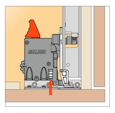
For side adjustment, it is recommended that the wheels on the clips are operated in the same direction, in order to maintain the correct alignment and movement of the runners.
