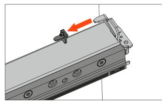
Insert the tilt adjustment levers AGLRXX3F, both right and left.
