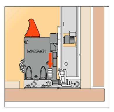
Rotate the white wheel towards the back of the drawer to adjust right. This operation is tool free.
