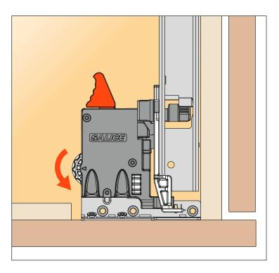
Rotate the white wheel (see drawing) towards the inside of the drawer to reduce the gap between the front and the side.
