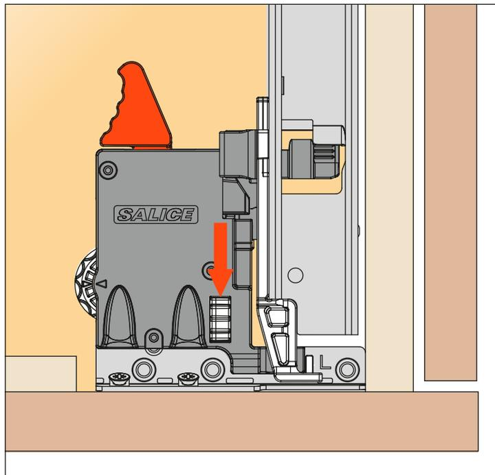
Rotate the white wheel towards the back of the drawer to adjust right.
