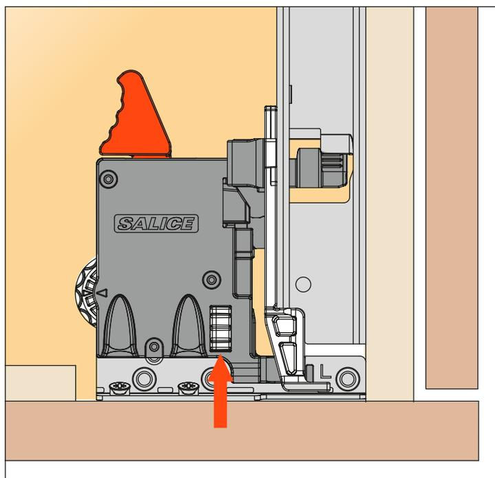
For side adjustment, it is recommended that the wheels on the clips are operated in the same direction, in order to maintain the correct alignment and movement of the runners.
