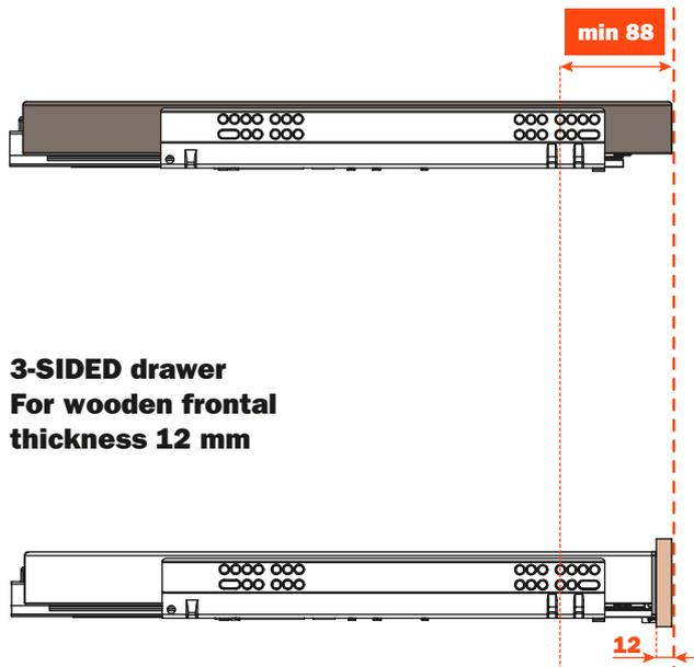
With the same side drilling, 4-sided drawers are **not frontally aligned** with 3-sided drawers with wooden frontal (19 mm thickness), as illustrated below.
