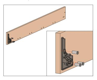
3. Insert and slide the front profile on the connecting elements Front profile support to cut to length, 90° mitre cut end, see pages 23, 25, 27.
