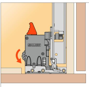
Rotate the white wheel (see drawing) towards the inside of the drawer to reduce the gap between the front and the side. This operation is tool free.
