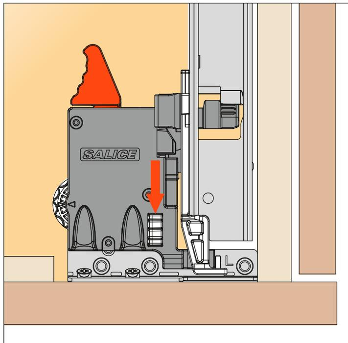
Rotate the white wheel towards the back of the drawer to adjust right.
