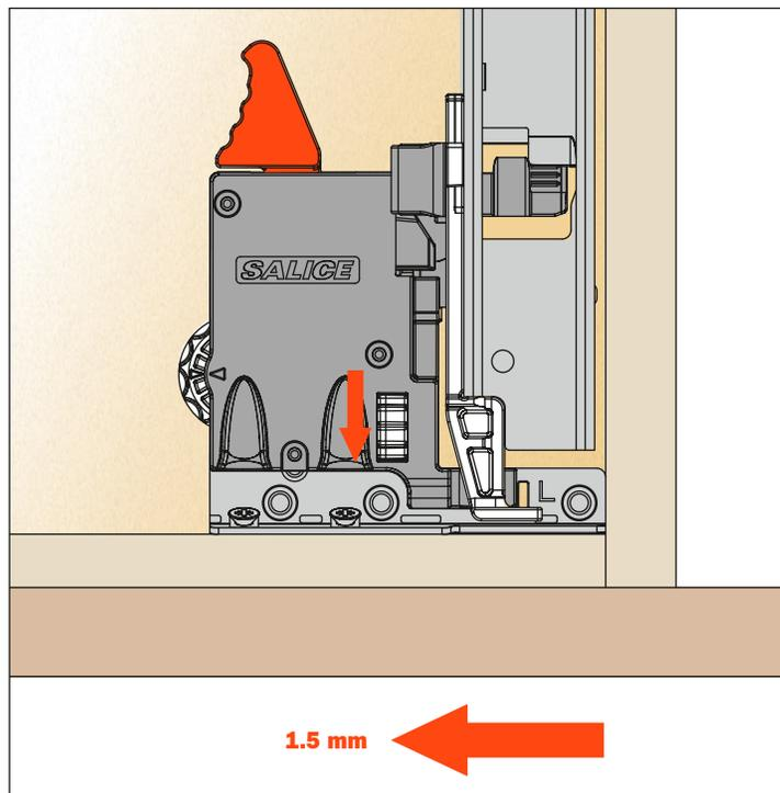
Rotate the white wheel (see drawing) towards the back of the drawer to adjust right.
