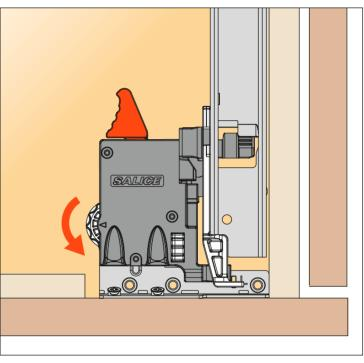
Rotate the white wheel (see drawing) towards the inside of the drawer to reduce the gap between the front and the side. This operation is tool free.
