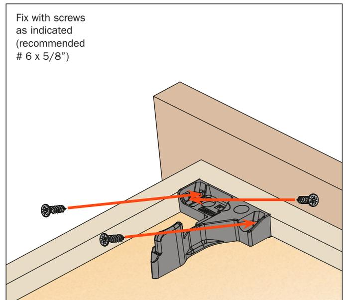
Use **drilling template** for accurate installation of the clips, see page 65.
