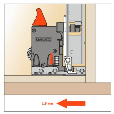
Rotate the white wheel (see drawing) towards the back of the drawer to adjust right. This operation is tool free.
