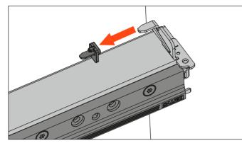
Insert the tilt adjustment levers, both right and left.
