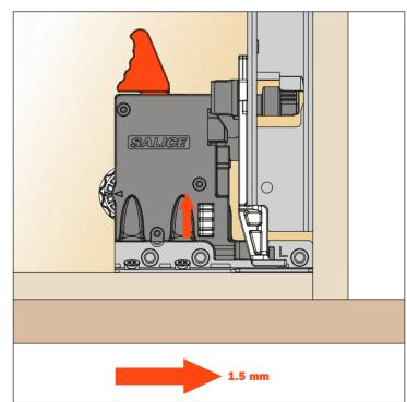
For side adjustment, it is recommended that both the adjusters on the clips are in the same direction, in order to maintain the correct alignment and function of the runners.
