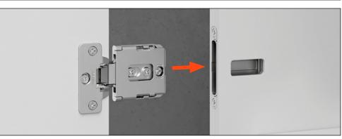
Once fully inserted, lock the hinge into place using the back cam
