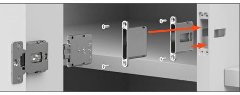
Fully insert the hinges into the holders
