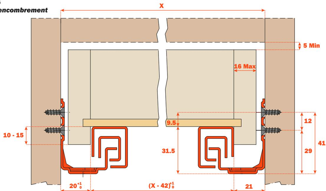
Note: the allowable drawer box width range is 41 mm to 42 mm.
