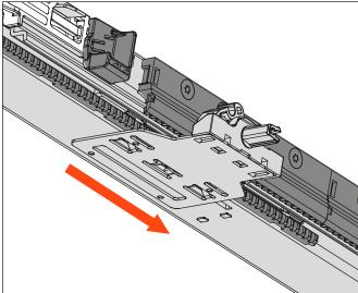
Fitting the driver pins to the runners
