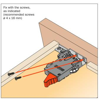
It is recommended to pre-drill the bottom or the frontal using the **SGD704UGXA drilling template**, see page 35.
