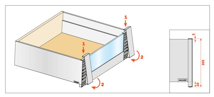
To correct any possible cutting errors of the panel, loosen and retighten the indicated screws  $% \left( 1\right) =\left( 1\right) \left( 1\right)$
