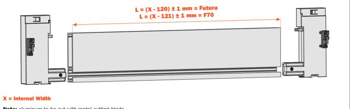
**Note:** aluminum to be cut with metal cutting blade Screws ø  $3.5 \times 20$  mm included. Can use #6 x 3/4" screws as a replacement
