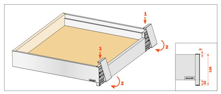
To correct possible cutting errors of the front profile, loosen and retighten the indicated screws
