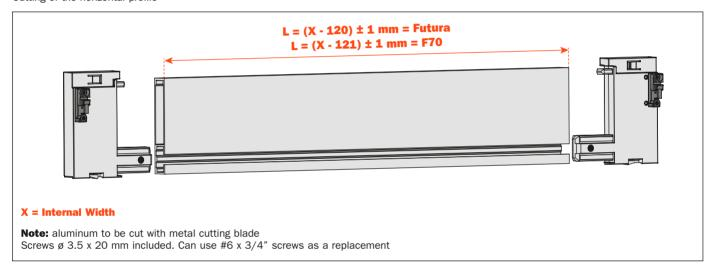
Insert the front panel adapters into the front panel and tighten the locking screws. Frontal fixings are already premounted.
