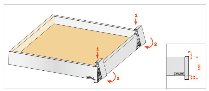
To correct possible cutting errors of the front profile, loosen and retighten the indicated screws
