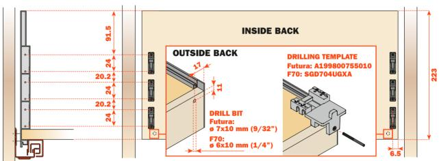
Note: Rear hook hole dimensions based on drilling with Salice drilling template A199800755010 with Futura runners or SGD704UGXA with F70 runners (see accessories, page 50).
