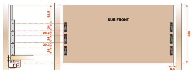
**BACK - Finished height & drilling dimensions**
