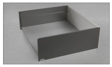
Lineabox metal sides, wood sub-front and back panel. Height of the side 178 mm - Internal height 149 mm. For use with Futura and F70 full-extension runners.
