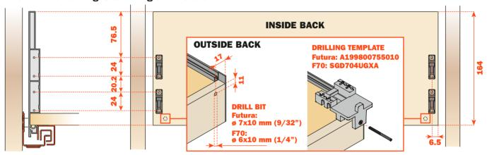
**Note:** Rear hook hole dimensions based on drilling with Salice drilling template **A199800755010** with Futura runners or **SGD704UGXA** with F70 runners (see accessories, page 50).
