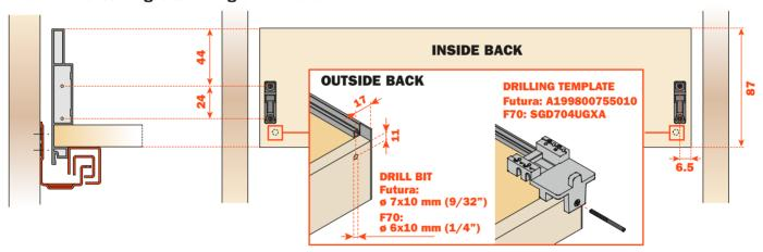
**Note:** Rear hook hole dimensions based on drilling with Salice drilling template **A199800755010** with Futura runners or **SGD704UGXA** with F70 runners (see accessories, page 50).
