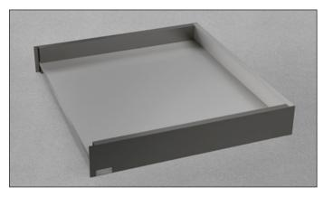
Lineabox metal sides, wood sub-front and back panel. Height of the side 75 mm - Internal height 46 mm. For use with Futura and F70 full-extension runners.
