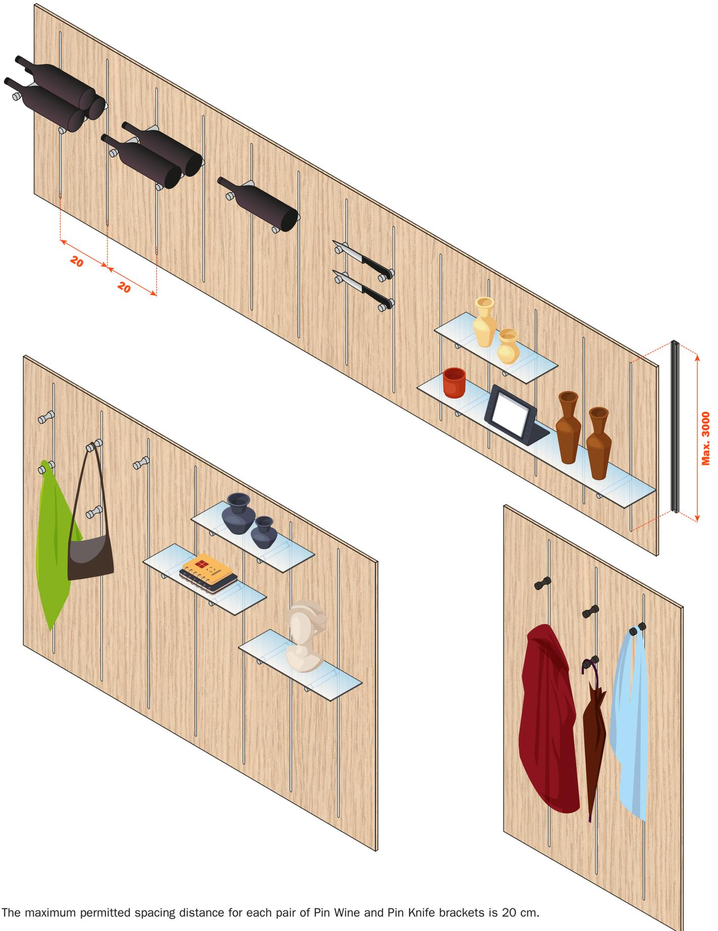
The maximum permitted spacing distance for each pair of Pin Wine and Pin Knife brackets is 20 cm.
