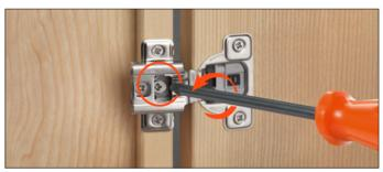
Side adjustment by eccentric cam for hinges: CU\_37D\_R - CU\_34D\_R = +2.5mm (3/32") / -1.8mm (1/16")  $CU_32D_R - CU_3AD_R - CU_3CD_R = +3mm (1/8") / -2mm (3/32")$
