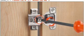
Depth adjustment by eccentric cam: + 2.5 mm (+ 3/32) / - 0.5 mm (- 1/64")
