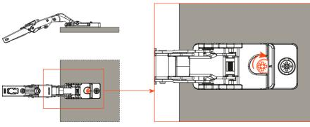
**3)** Rotate the locking cam. Use a#2 Pozi scewdriver.
