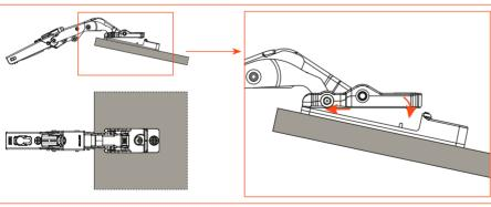
**2)** Locate the hinge onto the plate when it is attached to the door.
