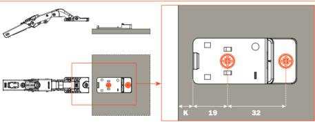
**1)** The hinge plate must be attached to the door with the included Euro screws.
