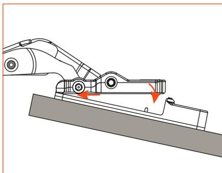
**2) Locate the hinge onto the plate when it is attached to the door.**
