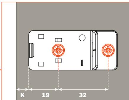
**1) The hinge plate must be attached to the door with the included Euro screws.**
