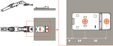
**1)** The hinge plate must be fixed to the door with the included screws.
