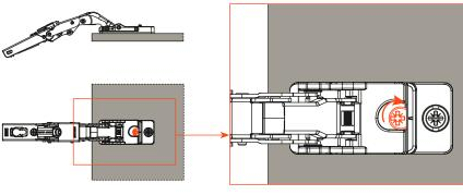
3) Rotate the fixing cam.
