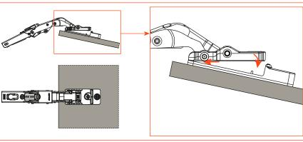
**2)** Locate the hinge onto the plate when it is fixed to the door.
