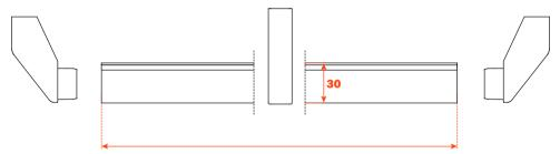
Length of the hanger rail = cabinet internal width L - 100 mm
