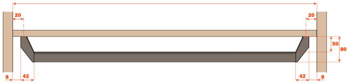
Centre support needed for hanger rails with length above 1200 mm or loads of more than 15 kg
