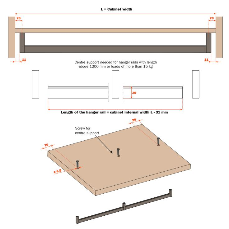
**YE80DAHA0133B** = Hanger rail for clothes, length 1000 mm **YE80DAHA0233B** = Hanger rail for clothes, length 1500 mm **YE80DAHA1233B** = End supports for hanger rail
