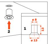
Insert the pins into the threaded inserts
