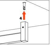
Tighten the grub screws
