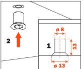
Insert the pins into the threaded inserts
