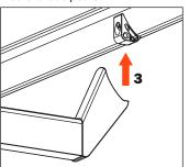
Screw-fix the rail-holders to the adapters
