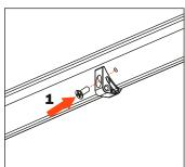
Insert the hanger rail into the rail-holders and insert them into the adapters
