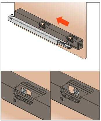
$\ensuremath{\mathsf{6}}.$  Secure the spacer in position using the front fixing screw
