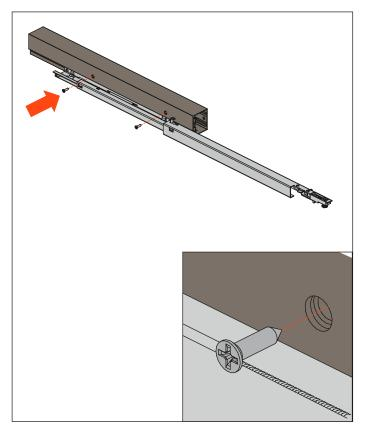
3. Screw-fix the spacer supports to the cabinet side
