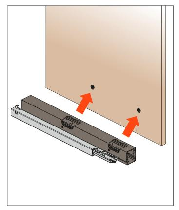
5. Slide the spacer backwards to locate the supports in their keyhole recesses
