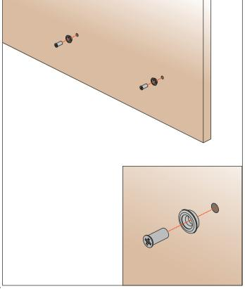
4. Position the spacer onto the supports
