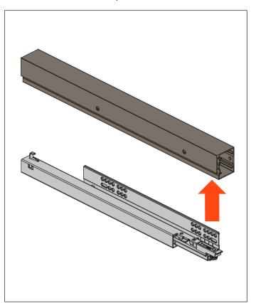
2. Fix the runner to the spacer using the screws provided
