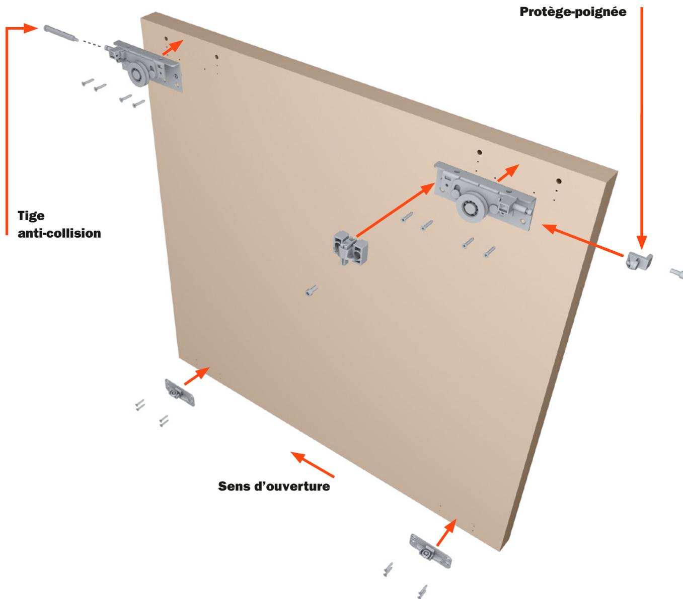
**Montage du mécanisme**
