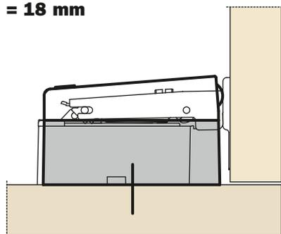
1 - Loosen one of the two fixing screws of the mounting plate.
