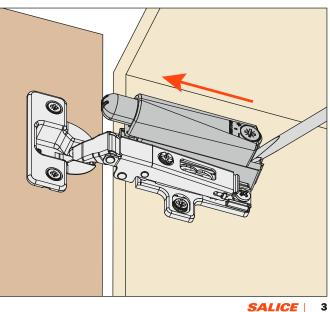
Fix the adapter in position using woodscrews.
