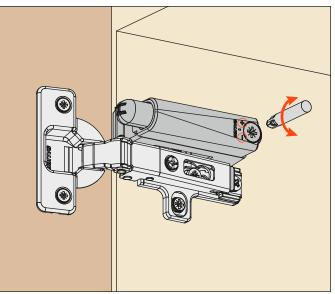
To remove the Smove piston assembly, insert a screwdriver in the indicated slot and prise it off.
