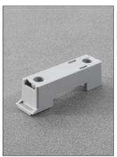
Screw-fix adapter for doors with "R" recess between 10 and 16 mm (half overlay). Smove works properly when it bears against the flange of the hinge. For this reason the appropriate adapter must be selected.
