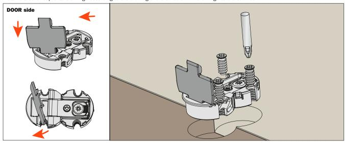
After fixing the hinge, make any adjustments required
