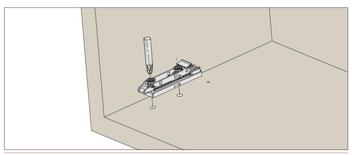
Fixing the hinge to the door
