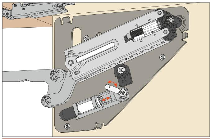
Adjustment of the opening angle of the door, by cam, from 80° to 92°.
