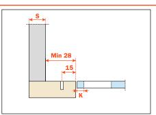
**Crampon hinges.** To be use only with Series 200 mounting plates for traditional assembly and drilling 28x32 mm.
