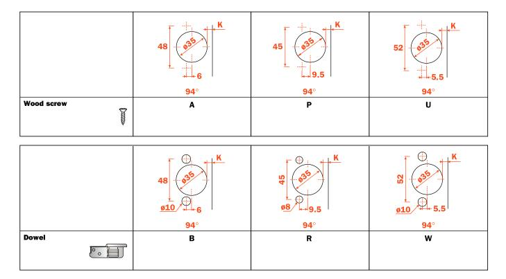
Use this table to identify the available drillings and fixings. Fill the third position of the hinge code number with the letter or the number corresponding to your choice. I.e.: C3\_BA99.
