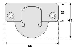
Constant "L" value of 0.7 mm (it does not change during side adjustment).
